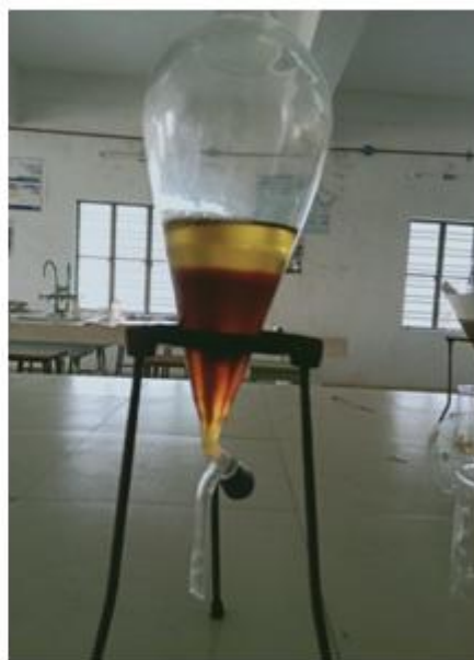
Biodiesel and glycerin separation
