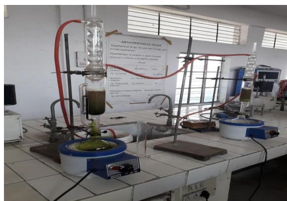
Fig.3. Preparation of leaf extracts using soxhlet apparatus
